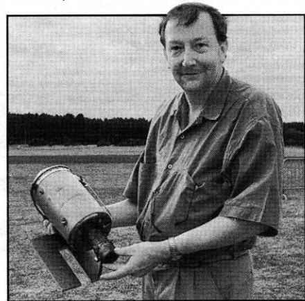
Joe Kuellen from Holland, of pulse-jet fame, has designed and constructed this gas turbine engine and is looking for an interested manufacturer. Any offers? We were unable to show the engine operating at Woodvale, none of the connectors would fit the propane gas bottle!
